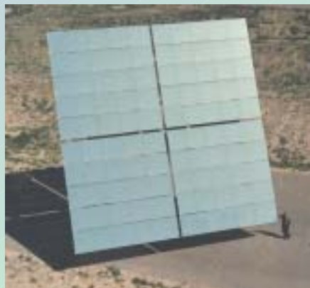
150 m 2 Heliostat (Advanced Thermal Systems)
